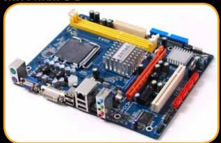
Experience a premium Microsoft® Windows® 7 Aero experience with the value ZOTAC G41. The ZOTAC G41 packs an Intel® G41 chipset with a Graphics Media Accelerator X4500 graphics processor for DirectX® 10 and OpenGL 2.0 compatibility. Support for 1333 MHz front-side bus processors ensures the ZOTAC G41 is ready to accept high-performance Intel® Core™ 2 Duo, Core™ 2 Quad, Pentium® and Celeron® processors for an unbeatable computing experience.
